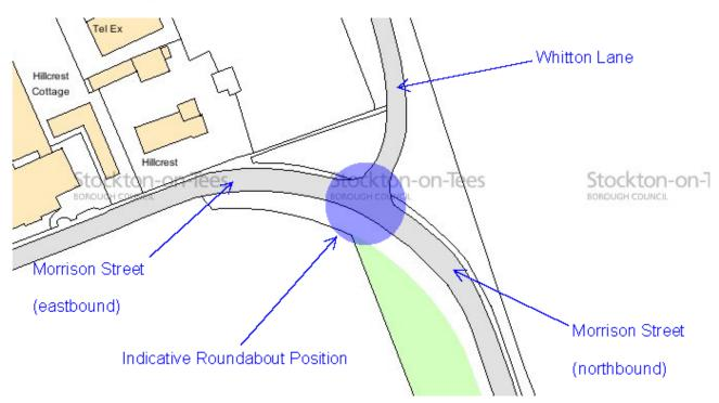
Setting aside the previously identified viability issues a review of the proposed Option1 roundabout layout, included at Appendix 1, has been undertaken by the Highways Transport and Design Manager and it is considered that, whilst this may be desirable, it is not achievable due to the alignment of Morrison Street in this location.
